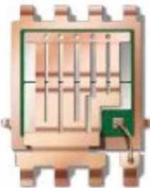
Cu Clip with Au Bump(S), Wire(G)
